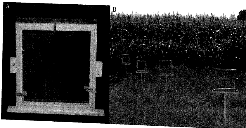
Figure 1 Wooden frame covered with two plastic plates for keeping orb-web spiders in the laboratory (A) and the exposure of spider webs at different distances from a maize field to determine pollen amounts in webs (B).
