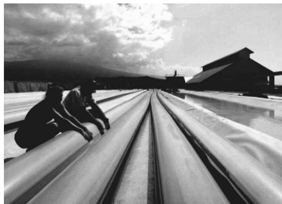
Fig. 4. The Mera Growth Module, a 25 000 l PBR.
